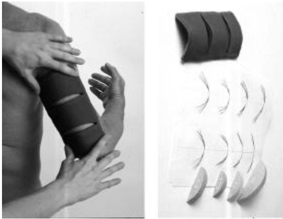
Figure 8, a shape-able tool used to map the arc of the triceps. Different peoples arcs are then mapped together to create an average concavity and width dimension to apply to wearable designs.
